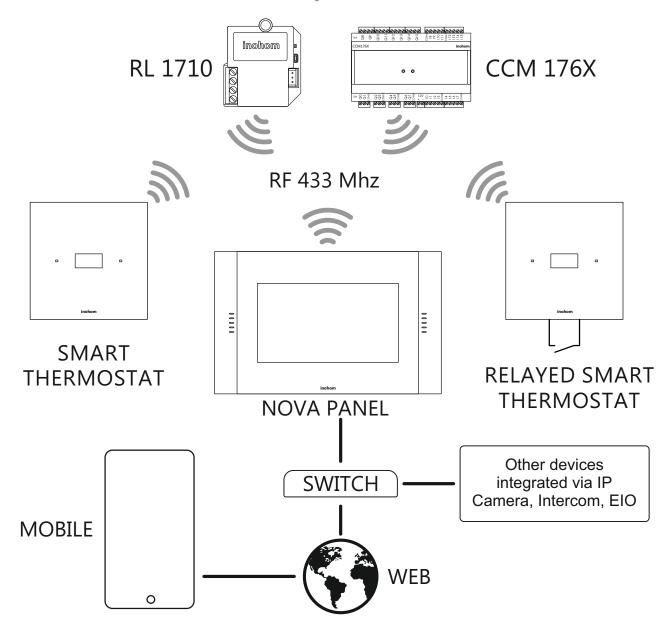
The devices use inohom communication protocol. Smart Thermostat can wirelessly communicate with other inohom products and can learn and switch output state values of other products.
