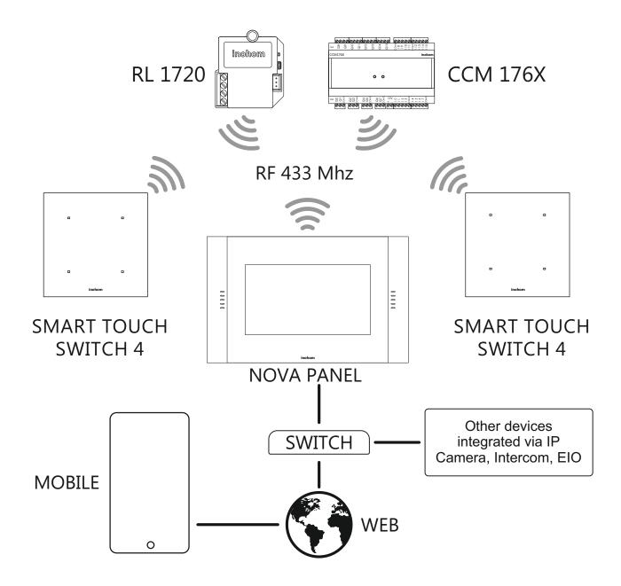
The devices use inohom communication protocol. Smart Touch Switch 4 can wirelessly communicate with other inohom products and can learn and change output and state values of other products.
