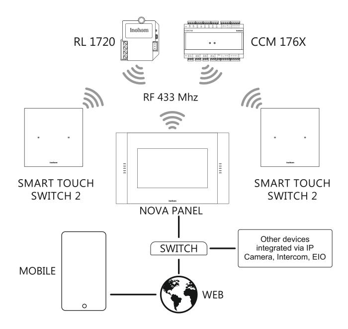
The devices use inohom communication protocol. Smart Touch Switch 2 can wirelessly communicate with other inohom products and can learn and change output and state values of other products.
