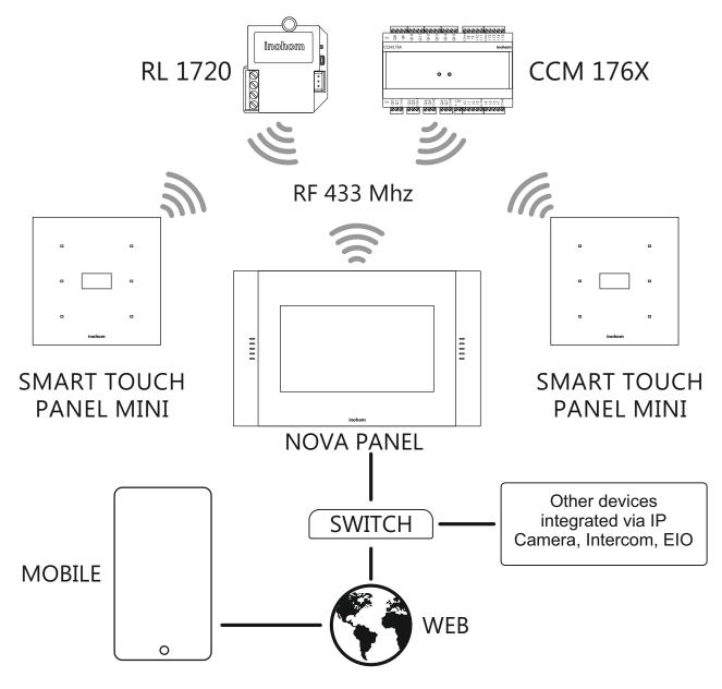
The devices use inohom communication protocol. Smart Touch Panel Mini can wirelessly communicate with other inohom products and can learn and switch output state values of other products.
