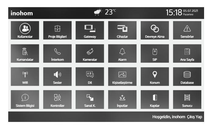
The commissioning of the inohom products after assembly is completed by the authorized inohom dealers and technical staff. Detailed management panel interface ensured communication and other settings between the devices.
